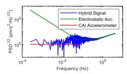
Figure 1: In green: PSD of an electrostatic accelerometer, Red: PSD of a CAI accelerometer, Blue: PSD of the hybrid signal.
